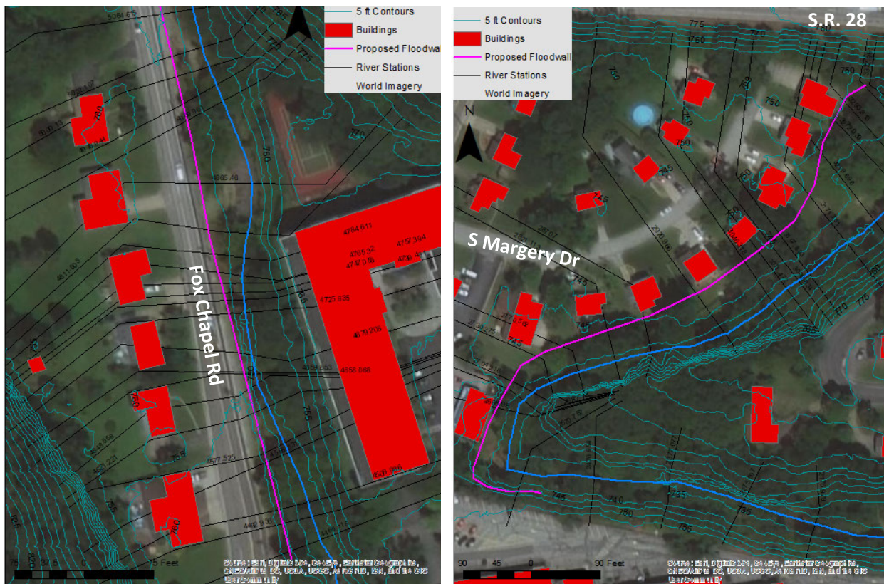
Fig. 3-3. Maps showing the extents of conceptual floodwalls 1 (left panel) and 2 (right panel).
