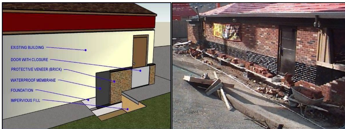
Fig. 4-10. Diagram (left) and photo (right) depicting veneer wall and waterproof membrane used in dry flood-proofing.
