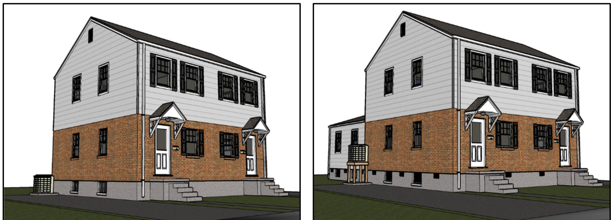
Fig. 4-4. Structure before basement abandonment, with basement and utilities located below DFE (left). Structure after mitigation, including installation of flood louvers, construction of addition to main structure to replace lost basement space, and elevation of HVAC unit (right).
